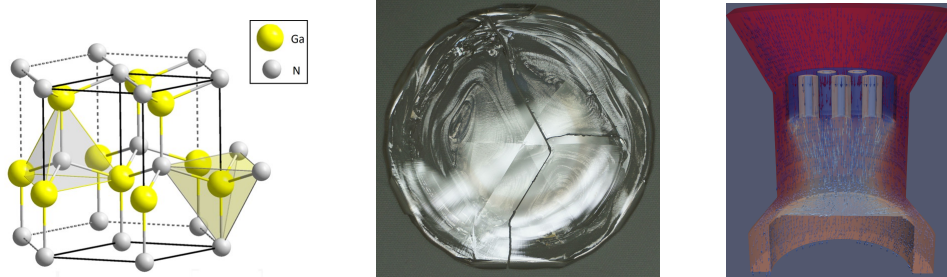
GaN's atomic structure, a crystal, and an HVPE reactor where it is grown.
